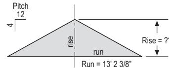
Remember: The PITCH of a roof equals its RISE in INCHES over a RUN of 12" thus a 4/12 roof has a SLOPE of 4". (when entering SLOPE always use inches) In Metric - pitch is expressed in millimeters over 1,000 millimeters of run.
